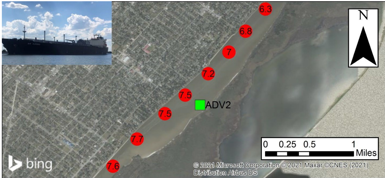
Figure 5-6 Vessel BW Kizoku Speed (kts) and Position Data From AIS Relative to ADV 2 Field Measurement Location
